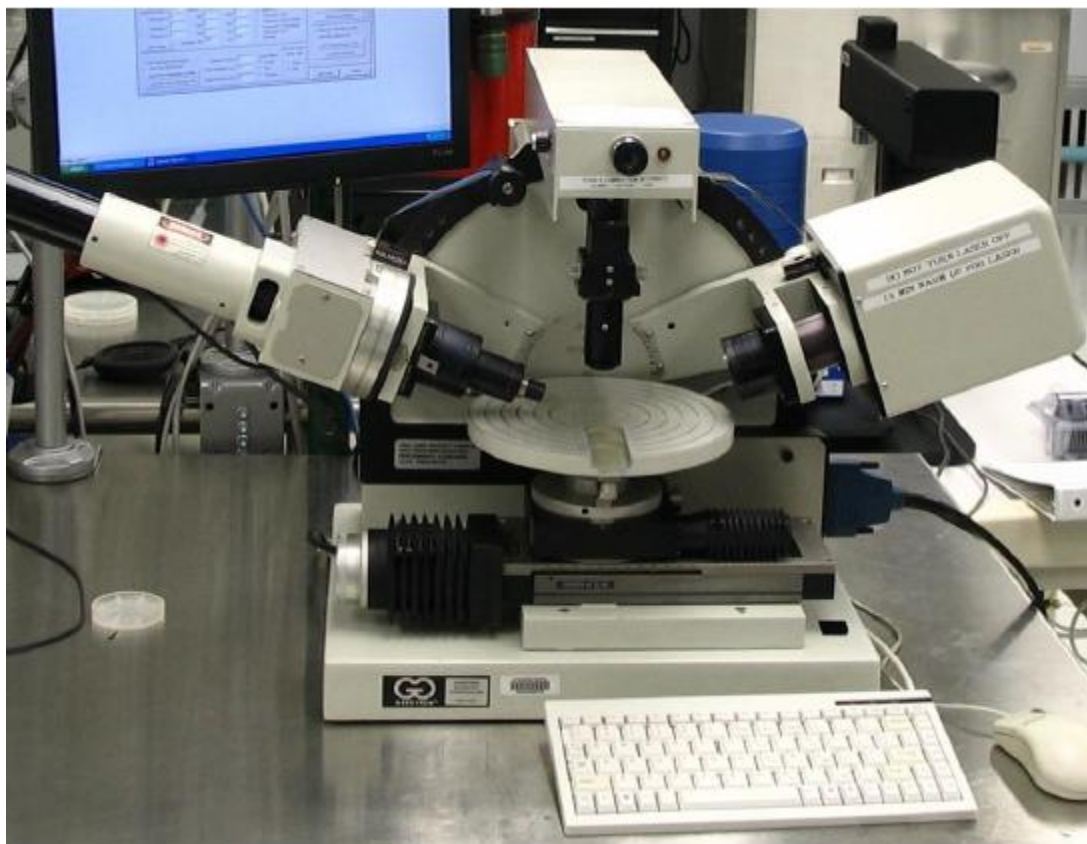
Figure I: Gaertner Scientific L115S-8 Ellipsometer
